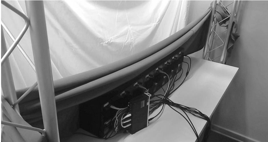
**Figure 5.3** Speaker array as set up for the study behind two acoustically transparent curtain, outside the subjects view.
